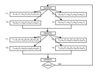
In this flowchart, during every iteration four threads concurrently compute the new values of a vector  $X_i$  as a linear function of  $Y_i$  values. Then the threads use a barrier synchronization.
